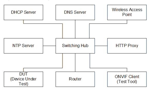
**DUT:** ONVIF device to be tested. Hereafter, this is referred to as DUT (Device Under Test).
