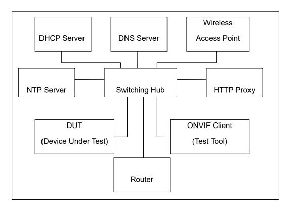
**DUT:** ONVIF device to be tested. Hereafter, this is referred to as DUT (Device Under Test).
