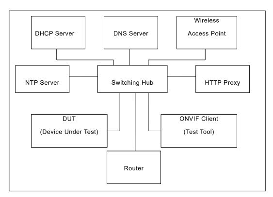
Figure 1: Test Configuration for DUT
