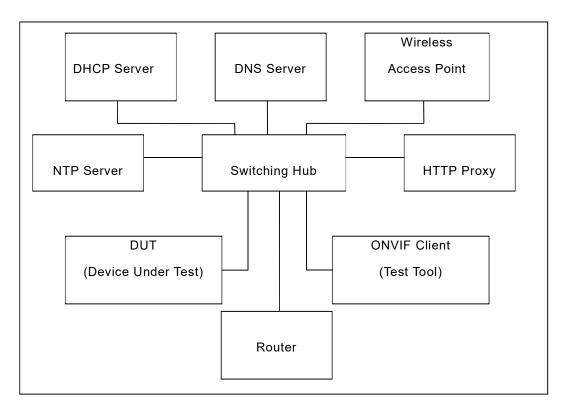
Figure 1: Test Configuration for DUT
